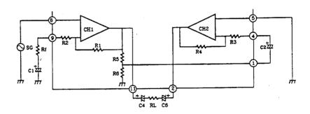
I )Fixed voltage gain (Pin 9 connected to GND directly)
